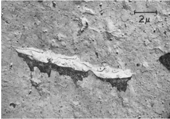
Fig. 7. Ozone crack profile in the 75/25 sulfur blend. Replicated at 10% strain.
