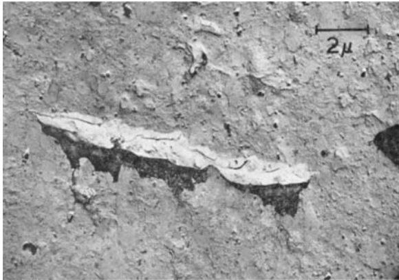
Fig. 8. Ozone crack profile in the 75/25 sulfur blend showing further evidence of crack jumping. Replicated at 10% strain.
